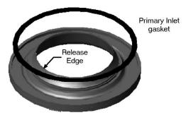
silicon RTV sealant. If the gasket is damaged or deformed where it might jeopardize a good seal, it can be reused once by pulling it free from the deflector and turning over, exposing an undamaged surface. Replace when both surfaces are damaged or deformed.
