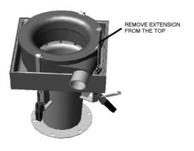
relatch. Repeat this first on the opposite latch then either adjacent latch and its opposite latch. Repeat starting with the first hook. Return again to the first hook and open it, leaving it hooked to the extension. Open the opposite latch, then open the remaining two latches and unhook the latch hooks from the Latch Hook Extensions (12). Remove the latch hook extensions from the deflector plate (13). The Maxi-Strip is now ready for complete disassembly.
